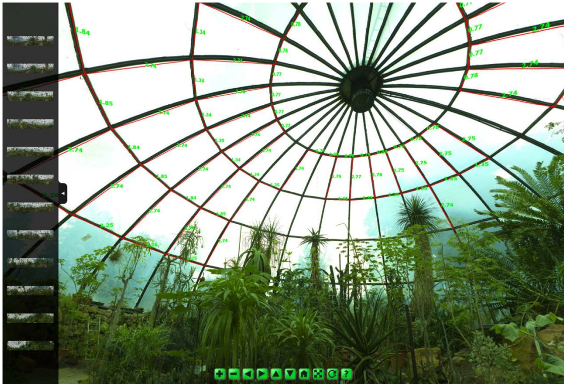
Fig. 6. 3D measurement and documentation with FODIS Measure3D of the Botanical Garden of Zurich.
